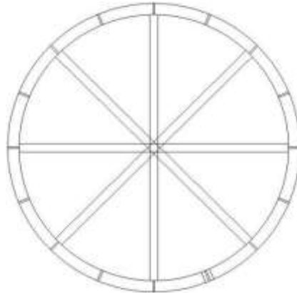
Figure 5.3.2-2 Reinforcement method at the horn upper outlet
