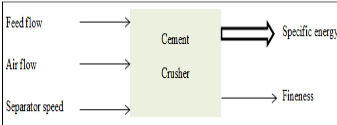
**Figure 2: Simplified schema of studied system.**
