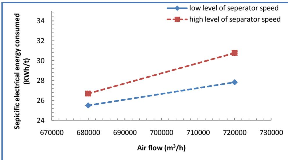
Figure 10: Effect of the interactions between the air flow and separator speed.
