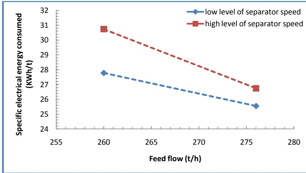
Figure 9: Effect of the interactions between the feed flow and separator speed.
