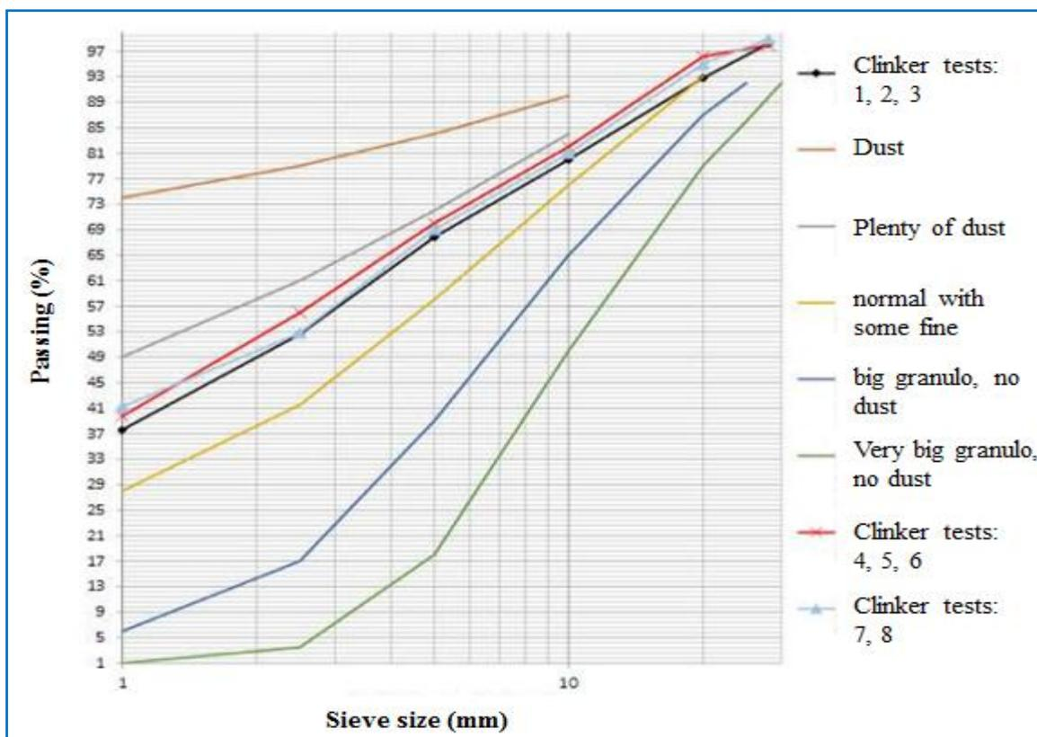
**Figure 3: Particle size distribution of test clinker.**
