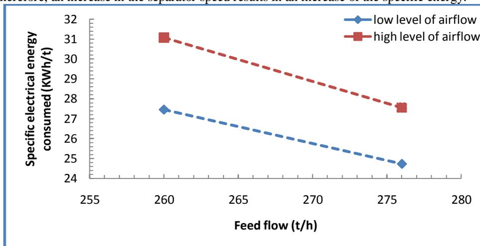
**Figure 8: Effect of the interactions between the feed flow and air flow.**
