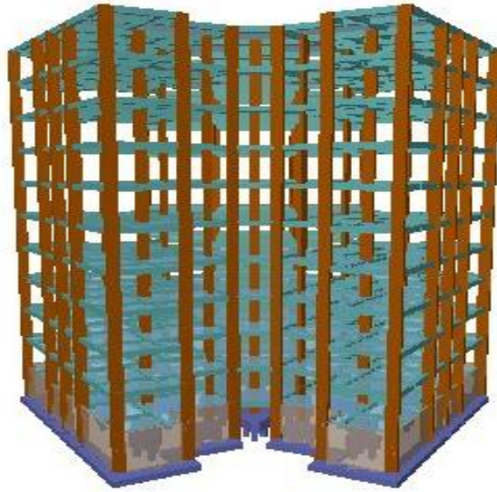
Fig. 10 Building Model with Shear wall in OGS storey
